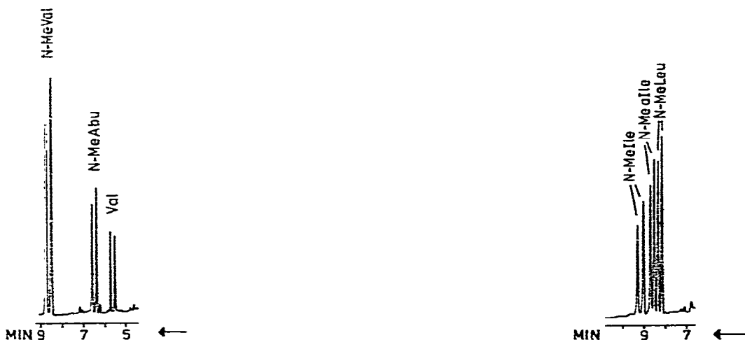
Fig. 1. Separation of (+)-3-methyl-2-butyl esters of DL-valine, N -methyl-DL- \alpha -aminobutyric acid and N -methyl-DL-valine on a 25 m \times 0.23 mm I.D. fused silica capillary column coated with CpSil-5. Column temperature, 90°C. Carrier gas, hydrogen (0.6 bar). Co-injection of 0.5 \mu l of MSTFA.
